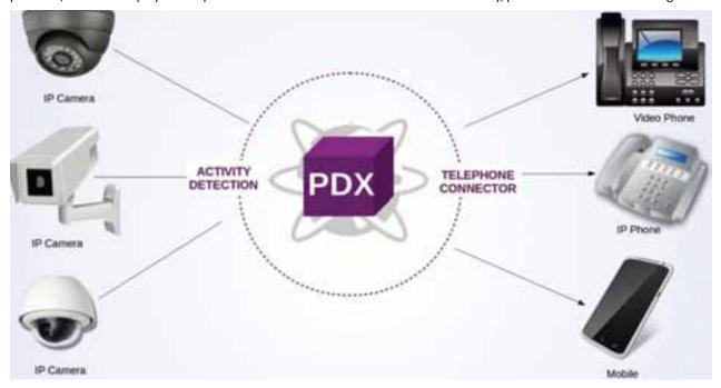
If the activity detection processor detects any activity, it can send an SMS, or email and also make calls to Mobile or Landline and play pre-recorded messages, depending on the premises, where activity was detected. An enormous cost-saving in terms of humans deployed to achieve the same results can be achieved. These methods may also be installed in locations, where the environment is hazardous for humans.
